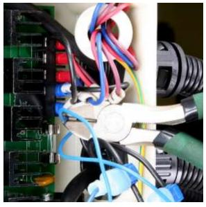
9. Replace the cable tie on the power leads using the new tie provided. 10. Replace the cover on the control box.
