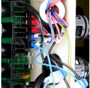
8. Cut the two wires within one inch of the terminals they are crimped into. It's OK to leave the bare ends exposed.
